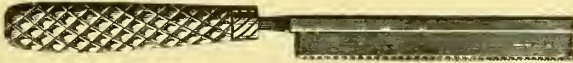
Fine saw, for cutting thin sections of bone and teeth, which are afterwards to be ground thinner on the hone and polished as described in § 95.
